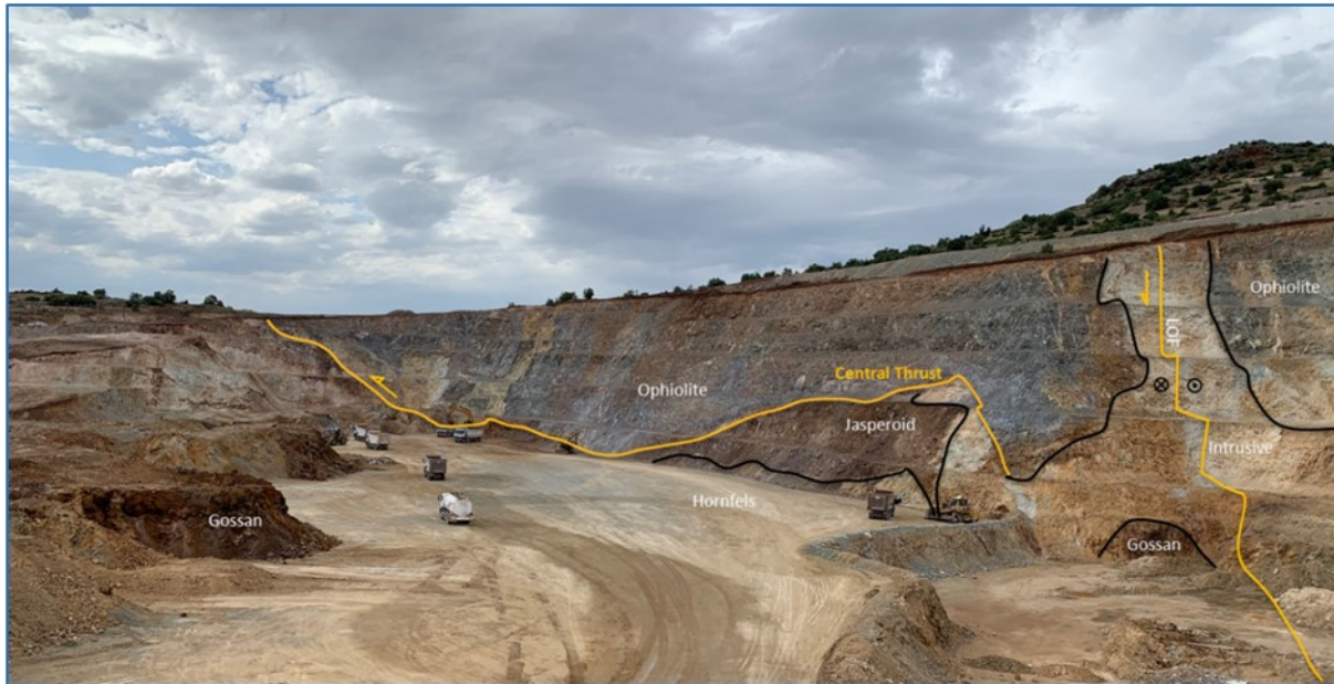
Figure 6.9 Geological Mapping within Çakmaktepe Central Pit
