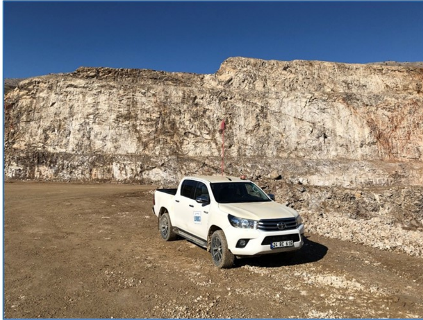
Figure 13.6 Typical 15 m Pre-Split at Çöpler Mine
